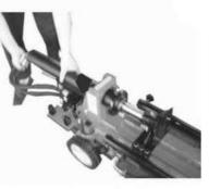
2.Lift the cylinder a bit.Take the cylinder bottom with two hands and rotate or move it from right to left and fit the screws to the cylinder holes.
