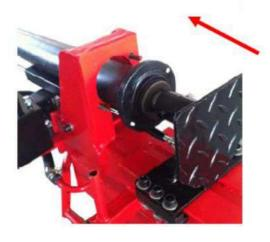
1.Push the cylinder to the opposite direction of the splitting wedge
