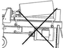
Break log in the direction of its growing grain. Do not place log across the log splitter for splitting It may be dangerous and may seriously damage the machine.
