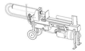
Following hydraulic oils or equivalent are recommend for the log splitter's hydraulic transmission system: SHELL Tellus 22 MOBIL DTE 11 ARAL Vitam GF22 BP Energol HLP-HM 22
